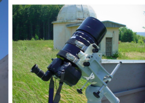
Photo-heliograph D=0.1 m Spatial resolution > 2000 km
