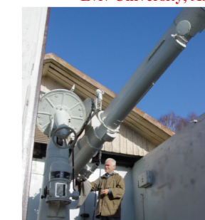
Chromosphere-photosphere telescope with an interference-polarization filter D=0.25 m
