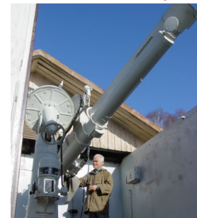
Chromosphere-photosphere telescope with an interference-polarization filter D=0.25 м
